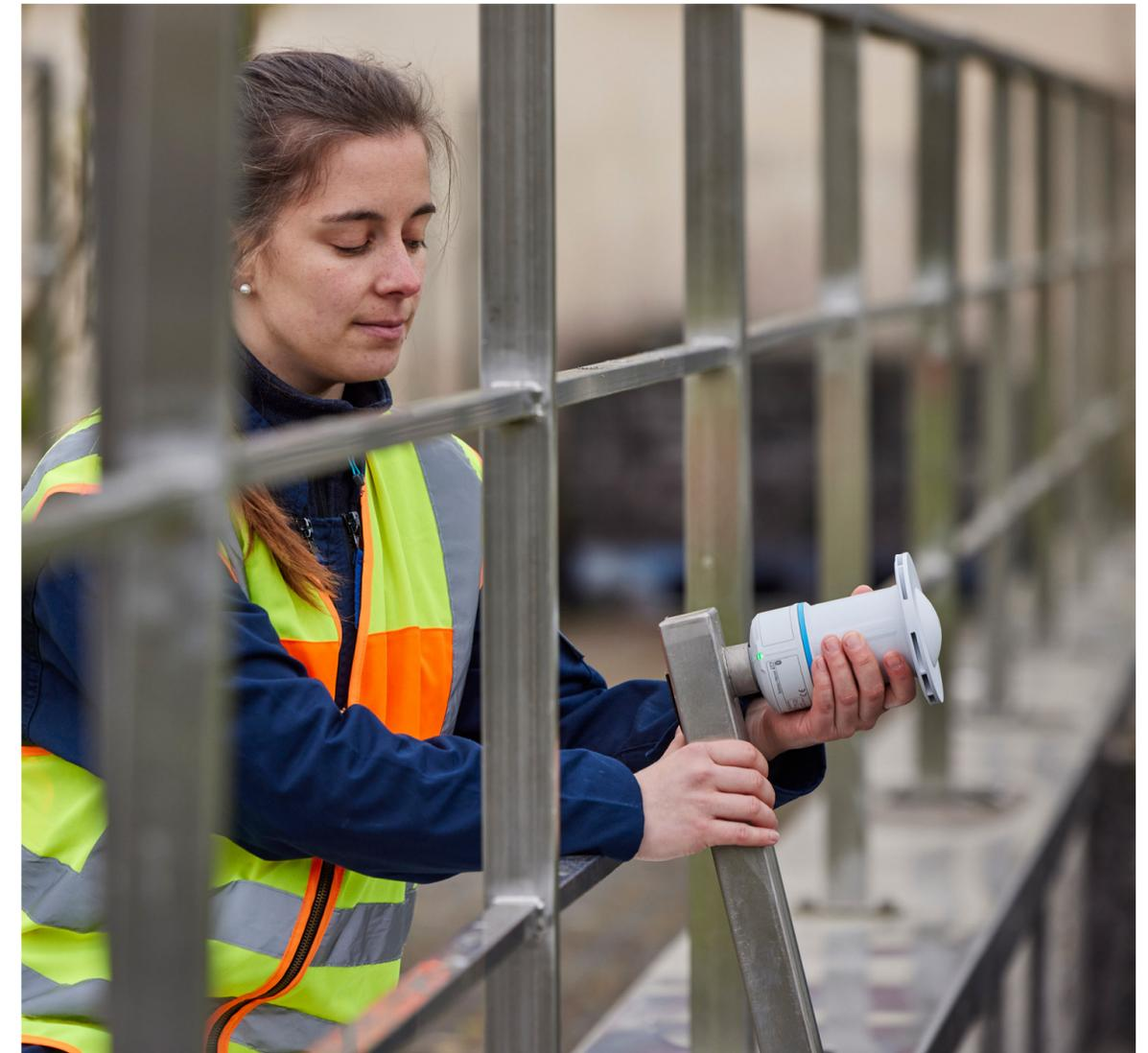
Heartbeat Technology allows documented, traceable and on-demand verification guided through wizard without process interruption. A device verification is performed in less than three minutes, without having to remove the device.
